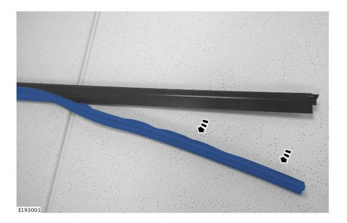
5. If installed, remove and discard the adhesive foam strip from the outer waist finisher.
