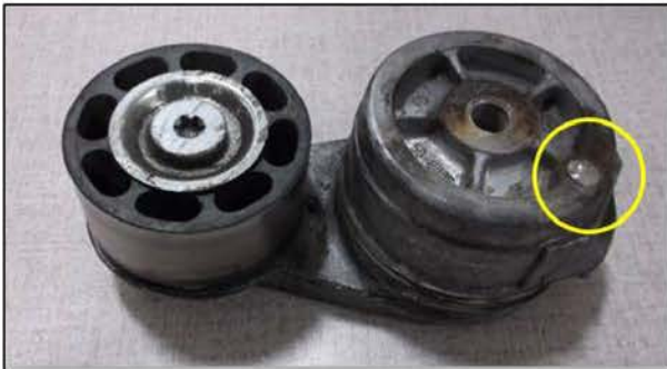
Figure 1: Belt Tensioner Locating Pin Failure
