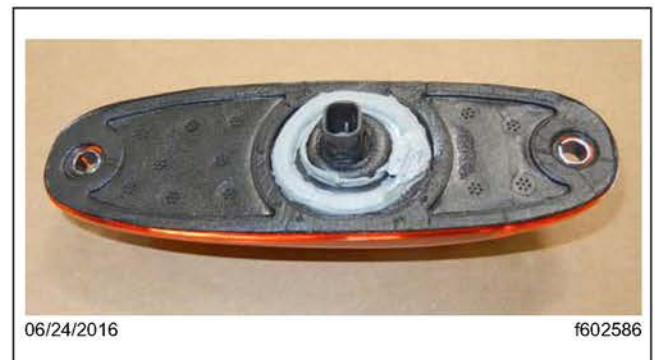
Fig. 2, Applying Sealant to Gasket
