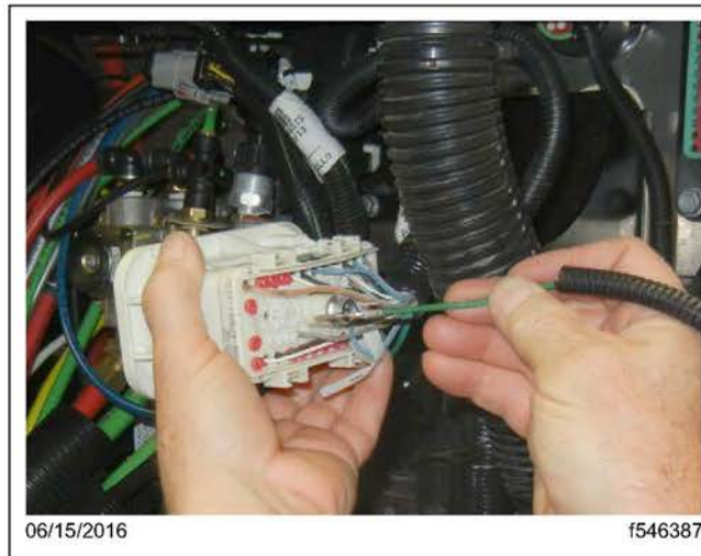
Fig. 4, Inserting Wire A06-91061-000 in to the Bulkhead Connector
