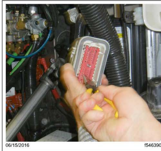
Fig. 2, Removing the Bulkhead Connector Terminal Lock
