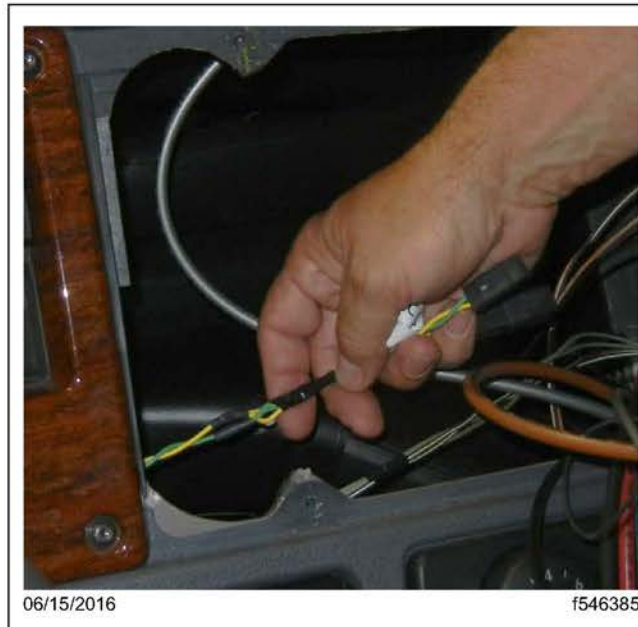
Fig. 8, Harness Wires Routed to the Auxiliary Instrument Panel
