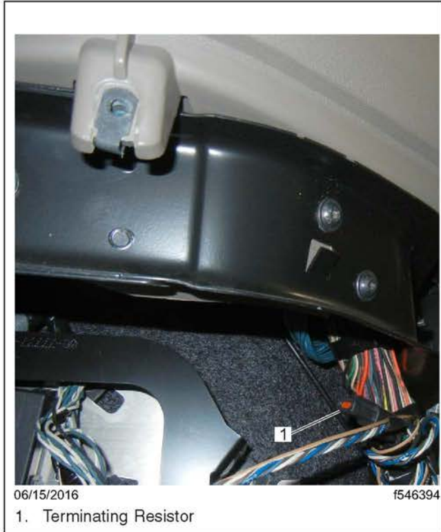
Fig. 9, Terminating Resistor Located Behind the Lower Center Cover
