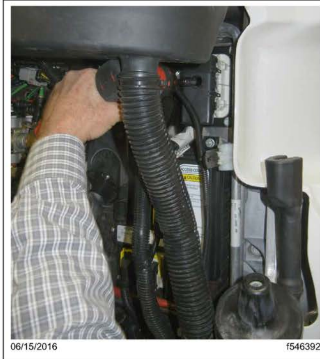
Fig. 1, Removing the Bulkhead Connector Mounting Bolt
