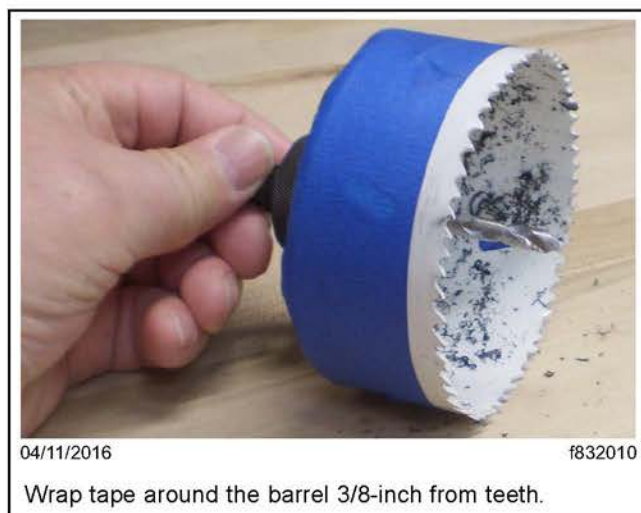
Fig. 4, Preparing the Hole Saw
