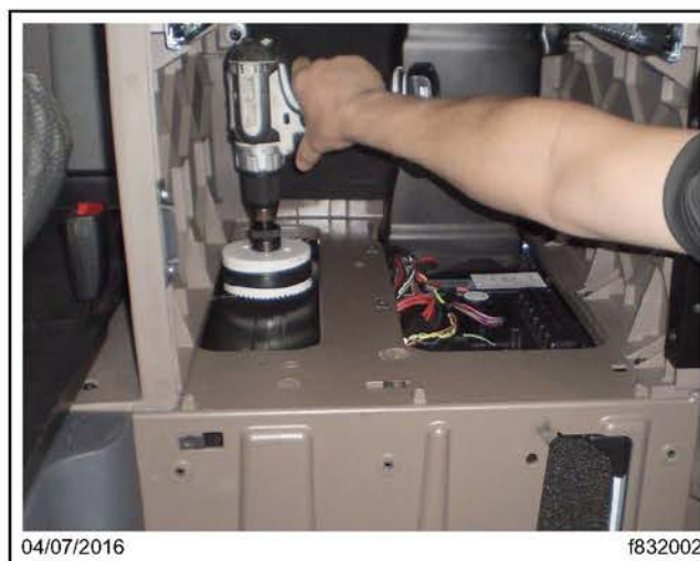
Fig. 6, Drilling the 4-inch Hole
