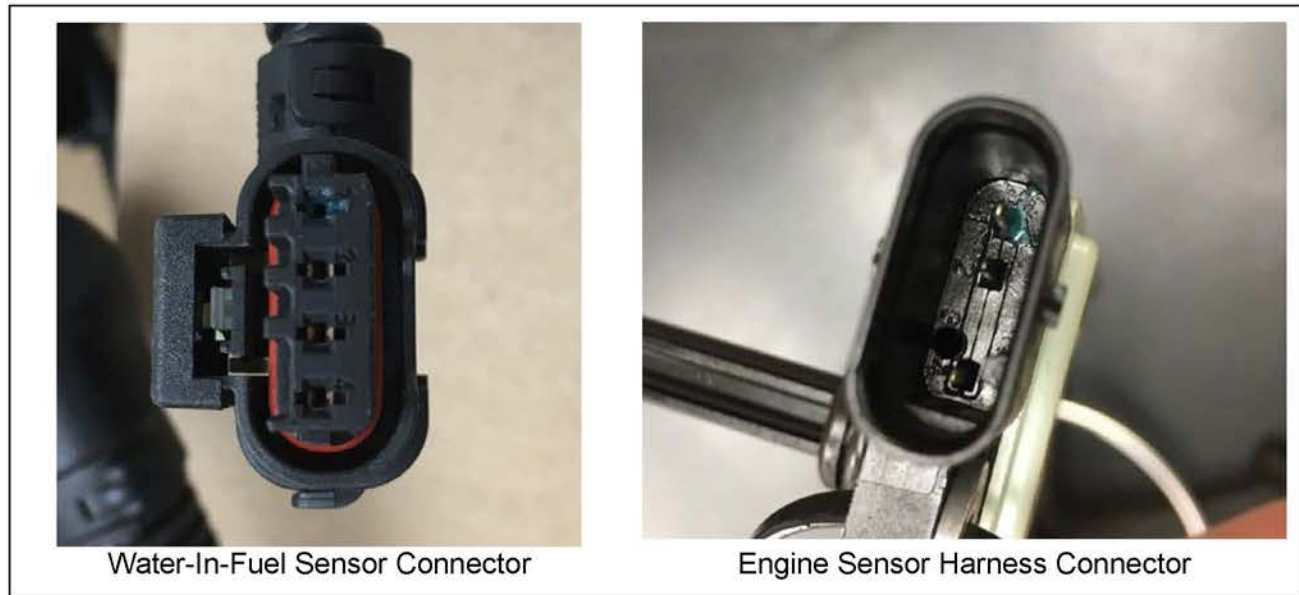
Figure 4 – Example of Damaged Connection at Water-In-Fuel Sensor Connection
