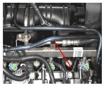
If the holding clip is missing, you will need retaining clip install one.
