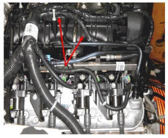
Inspect for a holding clip that secures the engine harness to the fuel line bracket. See Photo Below.
