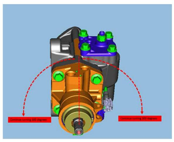
9. Rotate the steering gear input shaft 300 degrees from each side of the center of the input shaft.
