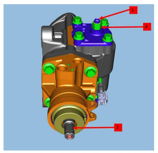
13. Tighten the steering gear pitman shaft lash adjuster nut (4) to 75-85Nm (55-63 lb ft).
