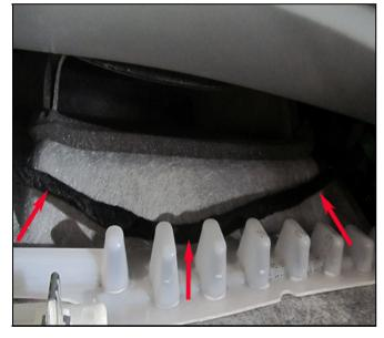
4. Reroute the RCDLR harness away from the opening for the rear HVAC duct on the headliner.
