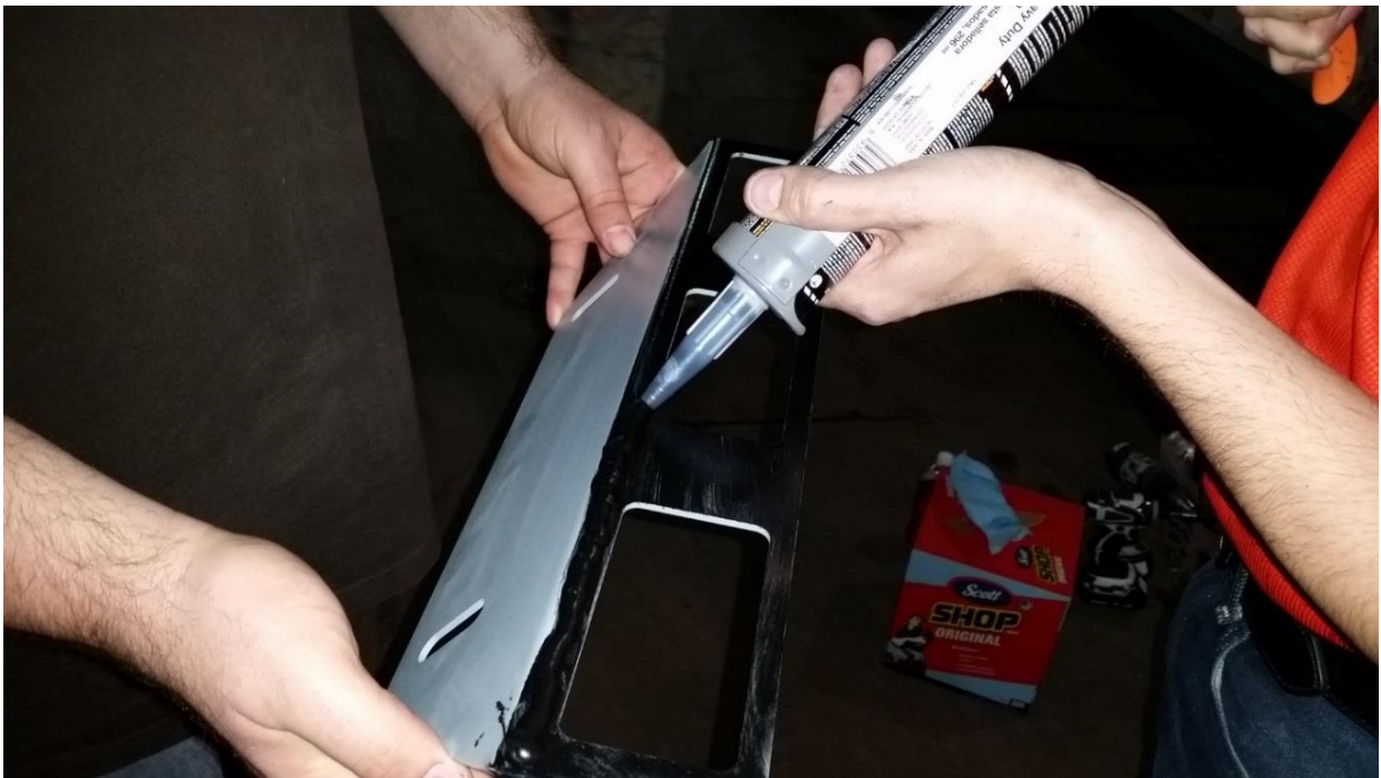
Figure 10: Sika adhesive application
