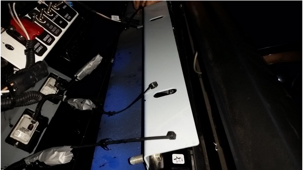
Figure 5: Cable ties taped to the connectors
