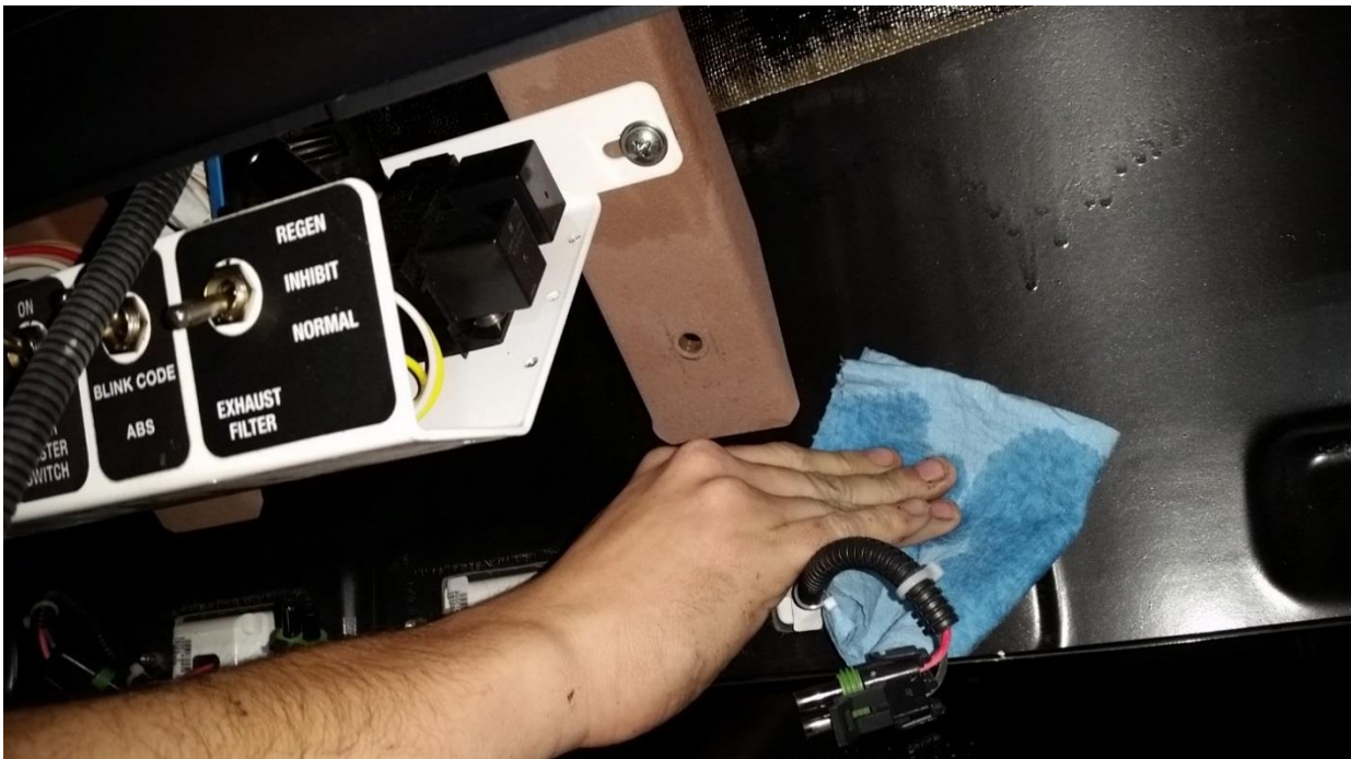
Figure 8: Apply Sika Aktivator/Cleaner on the bonding surface of the mask
