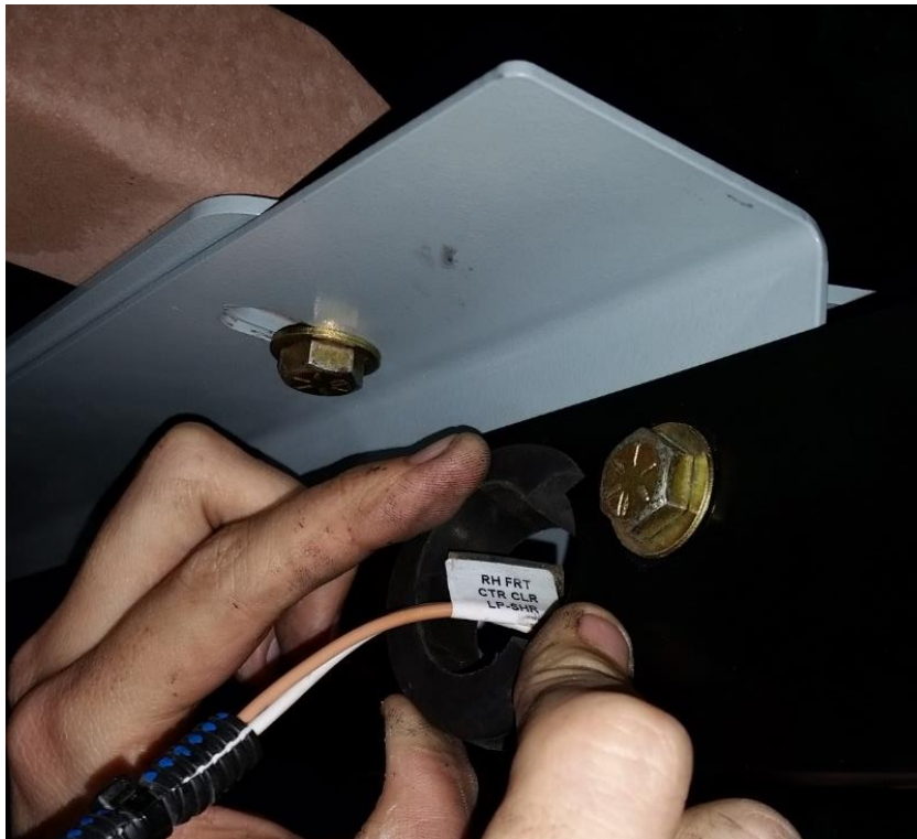
Figure 20: Re-connect the marker lights
