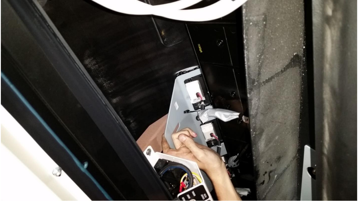
Figure 13: Front mask support bracket placement
