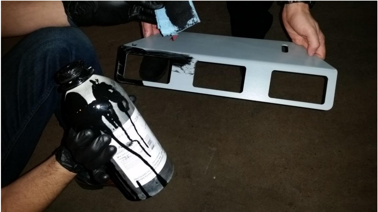
Figure 9: Apply Sika primer to the bracket
