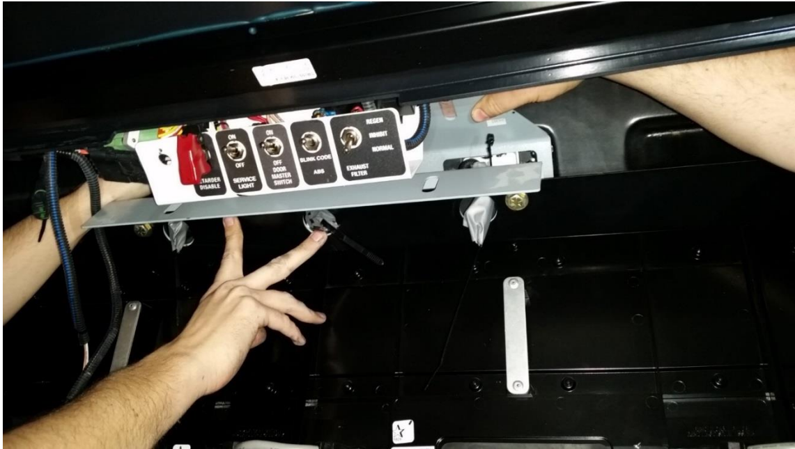
Figure 15: Place the destination sign closeout bracket in place
