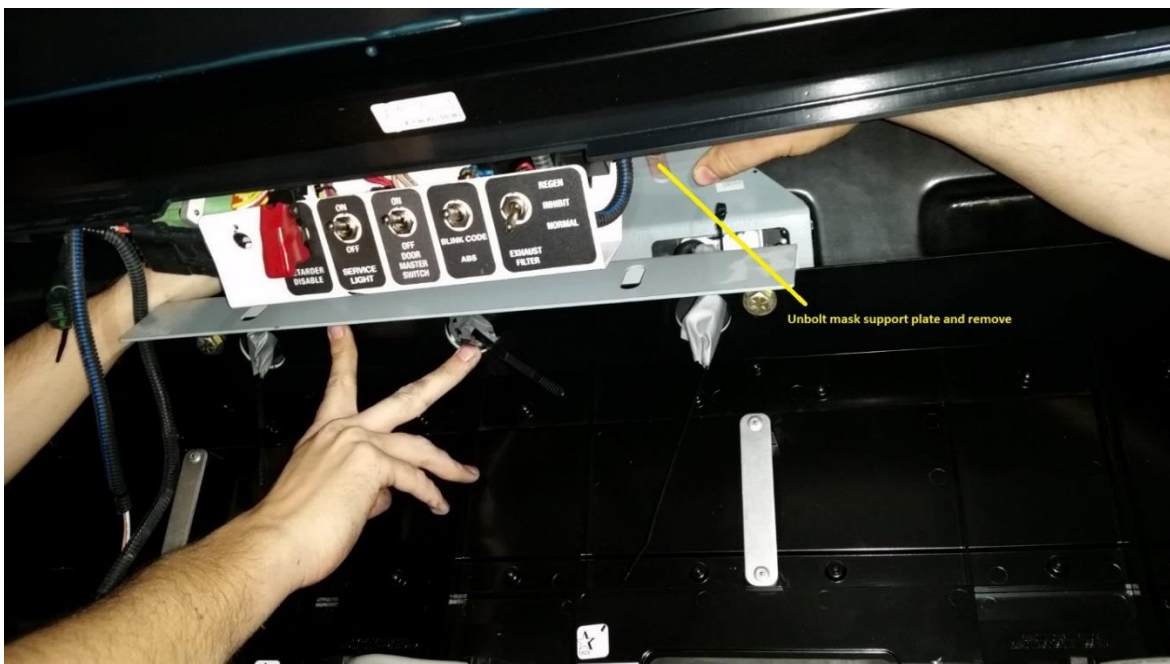
Figure 6: Remove the front mask support bracket
