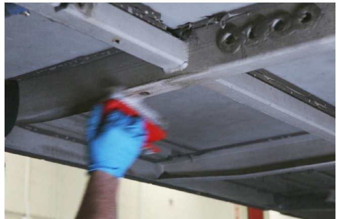
Figure 10 and 11: Spraying Krown Enviro Solve and scrub underbody structure with a brush
