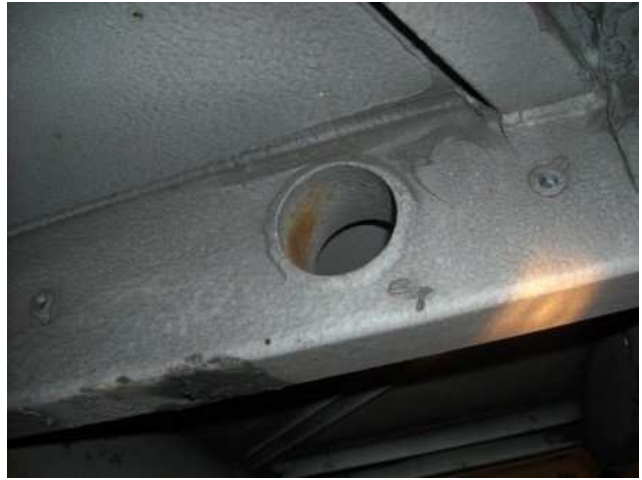
Figure 4 and 5: Example for corroded underbody surfaces
