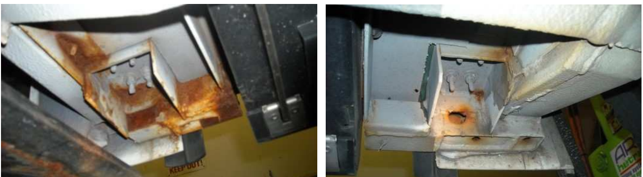
Figure 2 and 3: Example for corroded underbody surfaces
