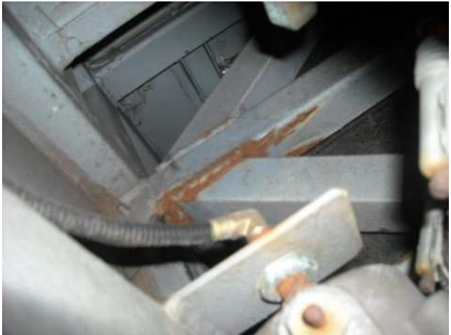
Figure 6 and 7: Example for corroded underbody surfaces
