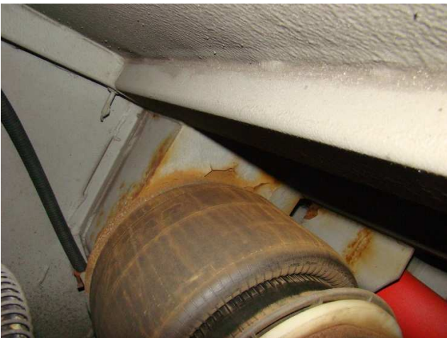
Figure 6 and 7: Example for corroded underbody surfaces
