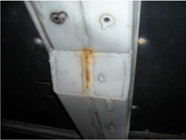
Figure 4 and 5: Example for corroded underbody surfaces
