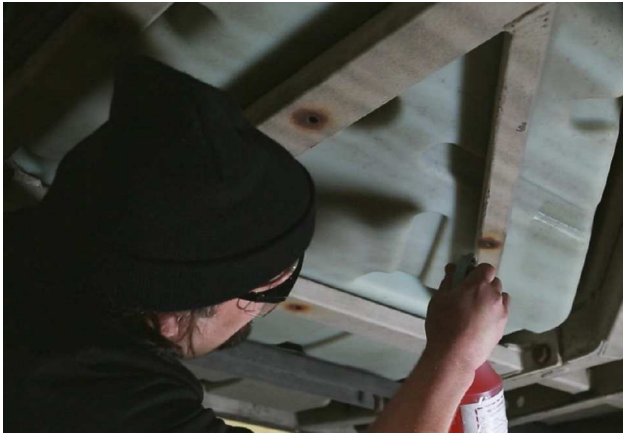
Figure 10 and 11: Spraying Krown Enviro Solve and scrub underbody structure with a brush
