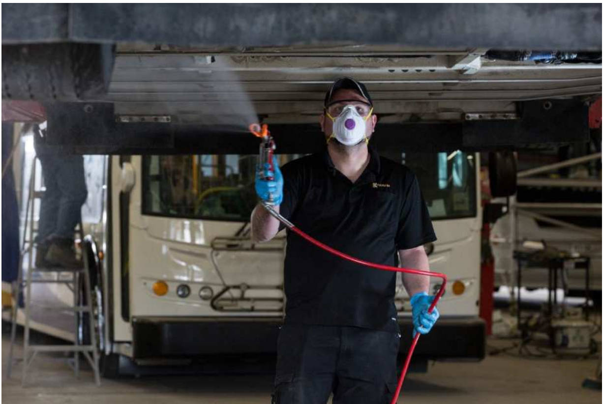
Figure 14: Application of T-40 to the entire underbody
