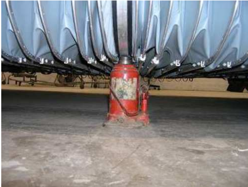
Figure 3: Lightly jack the bellow frame
