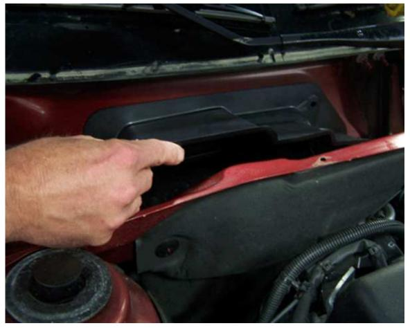
5. Apply the 143 Plastic Repair Adhesive above the foam on the backside of the deflector and install over the HVAC air inlet. The bead size should be 1/4"
