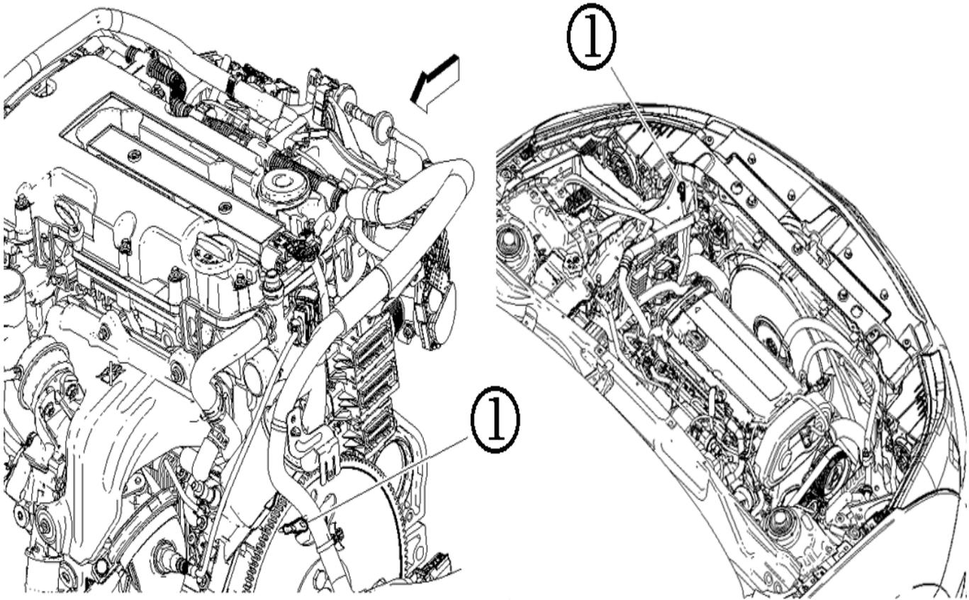
Inspect the G114 ground connections (1) and all other grounds on the engine. Check the engine compartment G114 ground connections (1), located on the left side, forward of the battery. Repair as needed.
