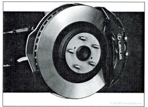
The 19-inch forged alloy wheels\* are paired with high-performance Brembo® front brakes, featuring massive six-piston aluminum calipers with 14.8-inch ventilated rotors with spiral internal fins for enhanced cooling.
