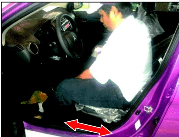
12. Confirm that the slide adjuster operates smoothly and verify the lock position timing is synchronized.
