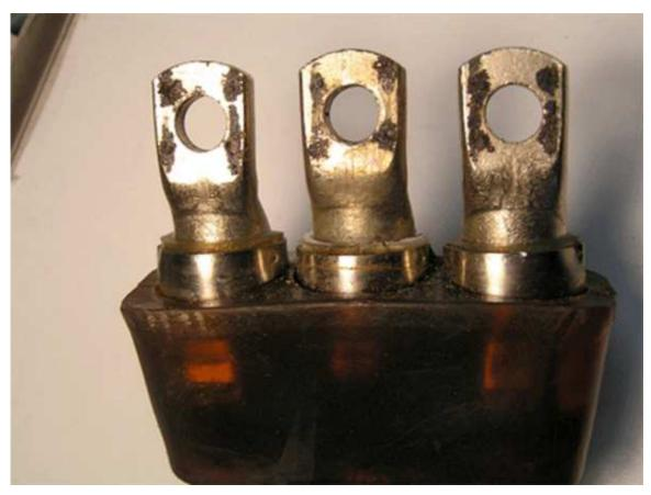
Terminals with signs of arcing/pitting that need to be replaced
