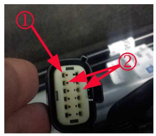
The next 2 pictures show what has been found with the terminals, this could be with either connector X160 or X161.
