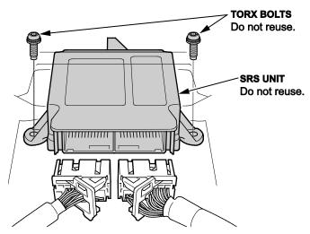
7. Install the new SRS unit using the new Torx bolts.
