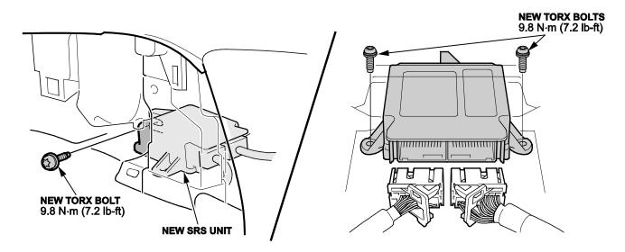
8. Connect the SRS connectors to the SRS unit by pushing the connector in and the lever moves to the locked position.
