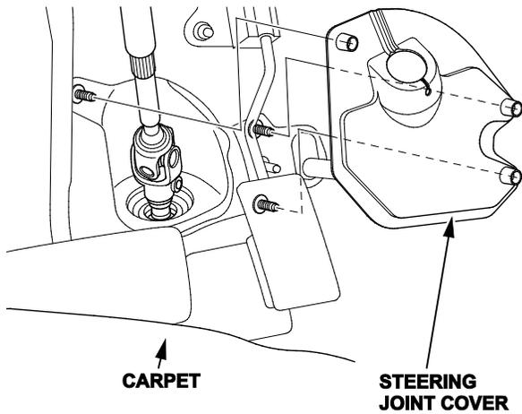
9. Remove the steering joint cover.
