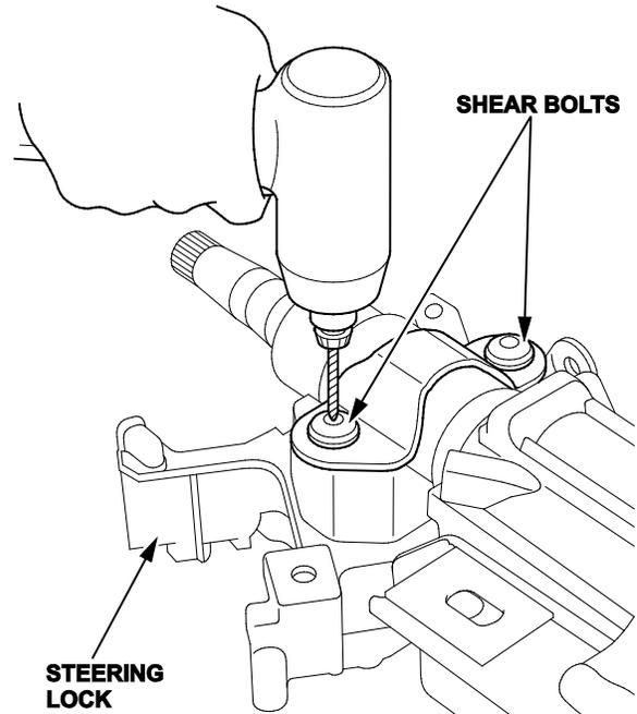
17. Remove the shear bolts from the steering lock, then remove the steering lock.
