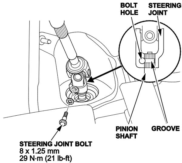
27. Pull on the steering joint to make sure the steering joint is fully seated, then tighten the steering joint bolt to the specified torque.
