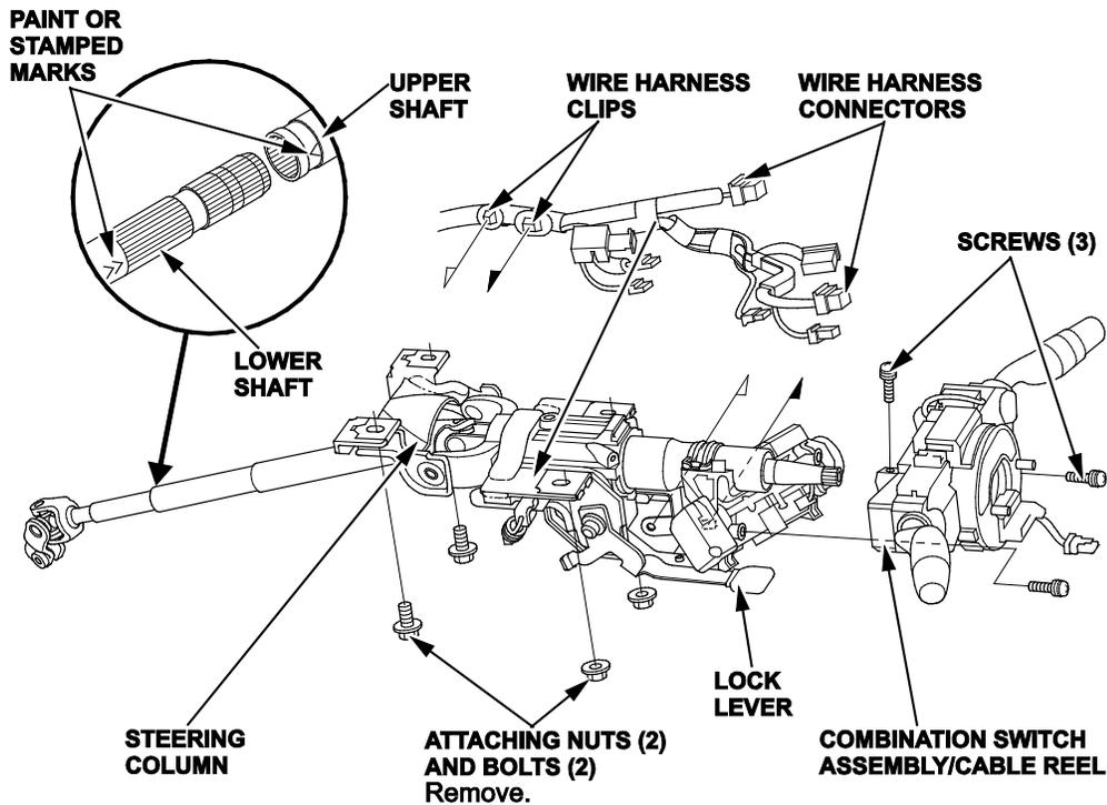
13. Remove the combination switch assembly/cable reel from the steering column shaft by removing the screws.
