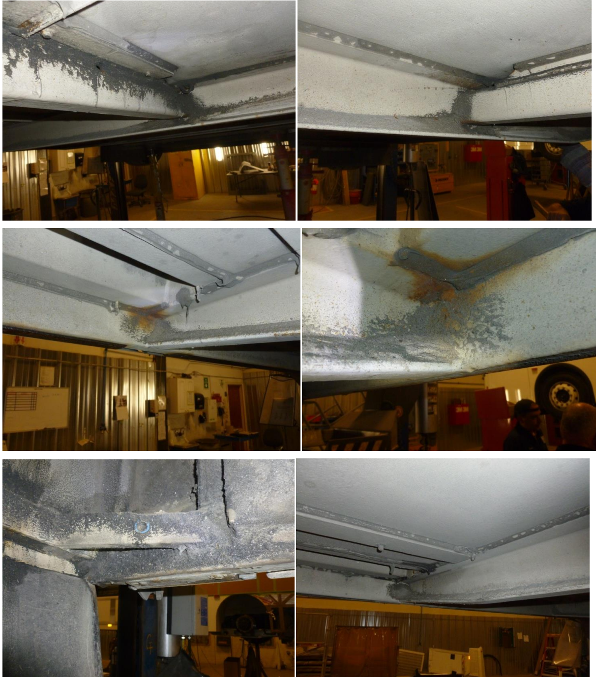
FIGURE 5: SHOWING TYPICAL EXAMPLES OF ROAD DEBRIS/SALT THAT NEEDS TO BE REMOVED.
