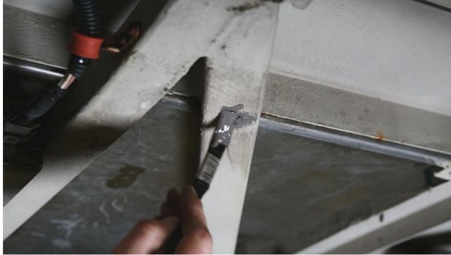
FIGURE 17: SHOWING PPG ZINC PRIMER APPLIED
