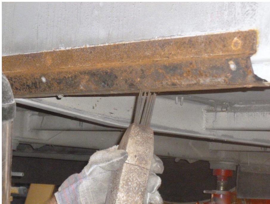
FIGURE 2B: AIR NEEDLE DE-SCALER USED ON OUTSIDE SURFACE OF LOWER IMPACT MOUNTING BRACKETS
