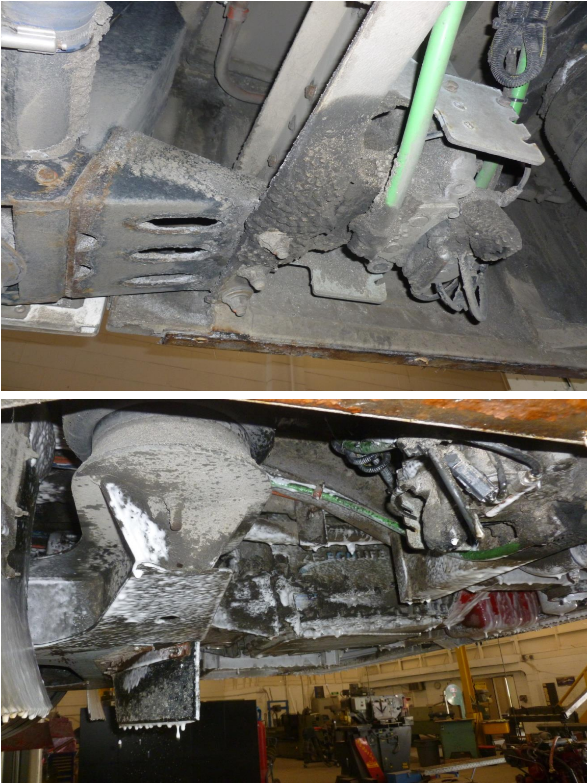
FIGURE 7: WHEN HEAVY DEBRIS, GREASE OR OIL STAINING EXISTS, USE OF A DEGREASER MUST BE USED.
