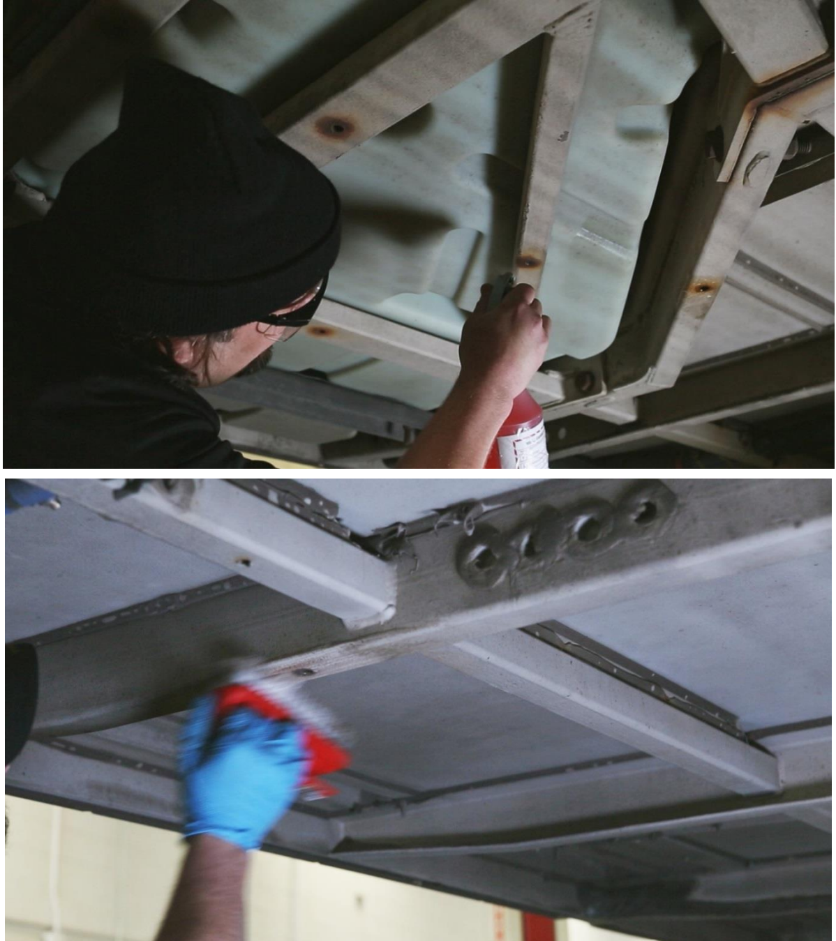
FIGURE 16: SHOWN APPLICATION OF THE KROWN ENVIRO SOLVE APPLIED, ABSORB FOR A 1 MINUTE AND THEN SCRUBBED OFF AS SHOWN. RINSE WITH WATER AND LET DRY.
