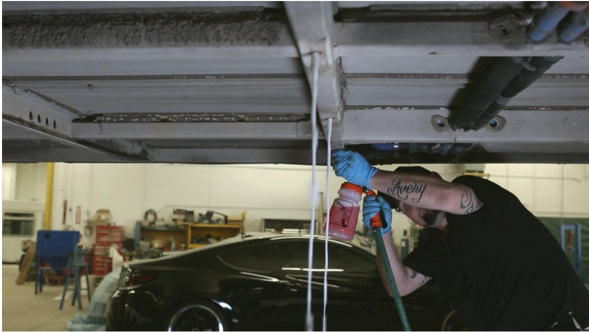
FIGURE 10: APPLICATION OF SALT ELIMINATOR BEING APPLIED INSIDE TUBES TO FLUSH OUT DEBRIS AND CALCIUM BUILDUP
