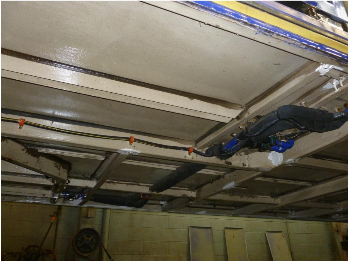
FIGURE 23: SHOWN VIEW OF THE UNDERSIDE SPRAYED WITH T-40. “WET” LOOK IS THE FINAL PRODUCT SHOWN ON THE UNDERSIDE.
