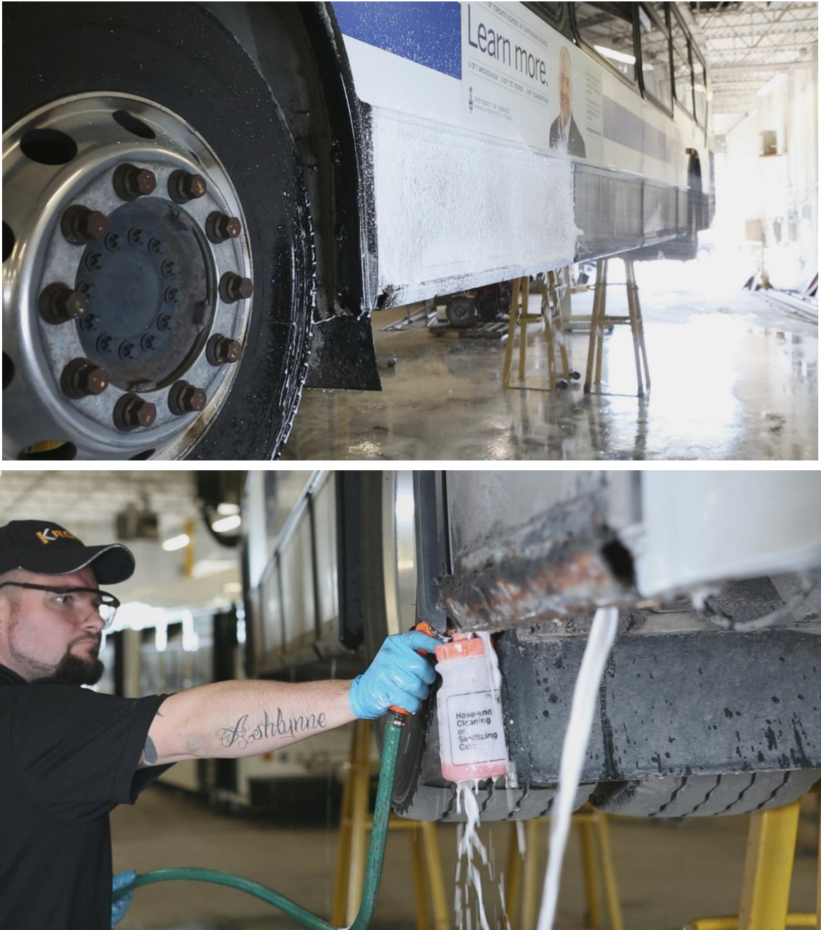
FIGURE 8: SHOWN THE APPLICATION OF THE SALT ELIMINATOR SPRAYED ON THE PANELS AND LOWER IMPACT PANEL BRACKETS/RAILS.
