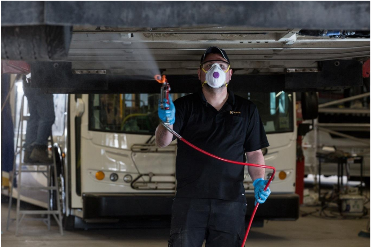
FIGURE 22: SPRAY T-40 ON THE UNDERSIDE OF THE BUS.
