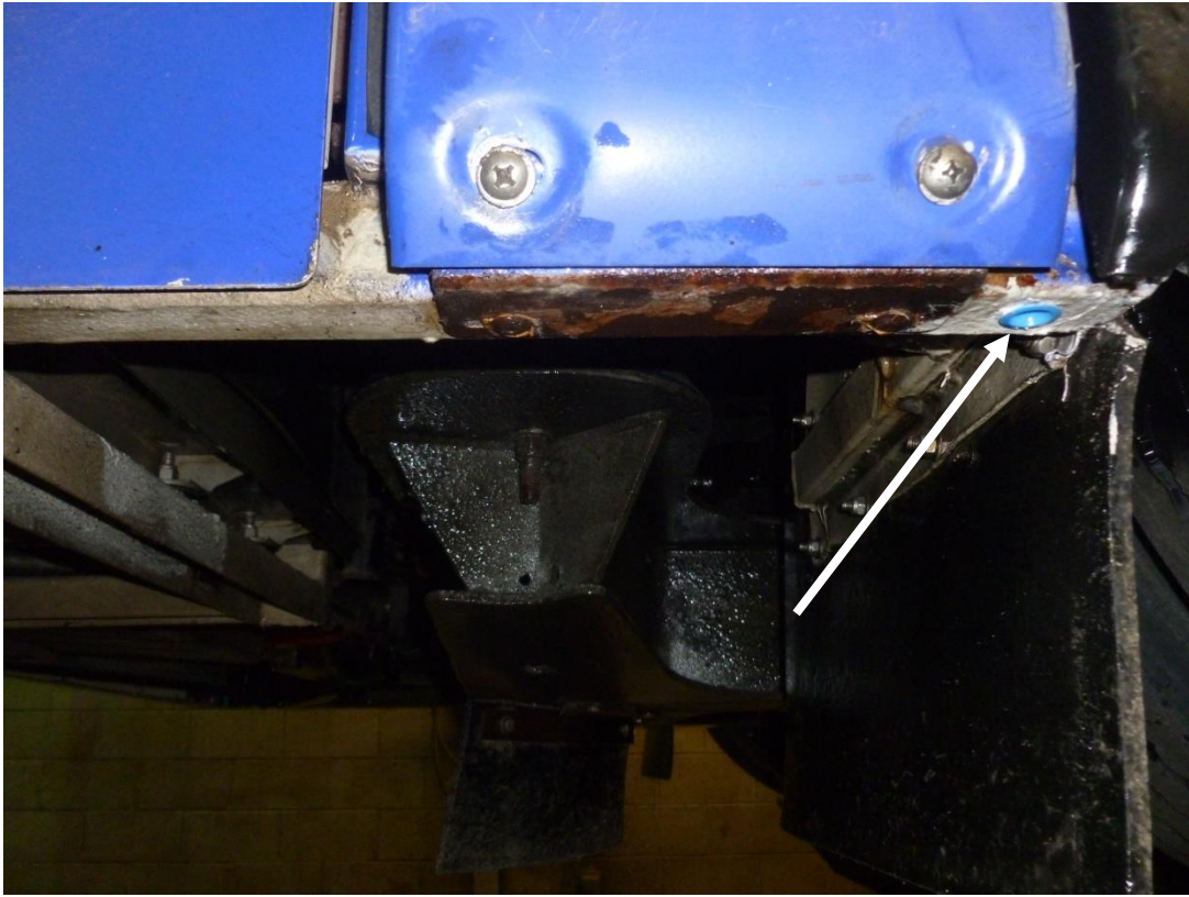
FIGURE 24: SHOWN THE 1/2" HOLES PLUGGED WITH LITHIUM GREASE & BLUE PLUG
