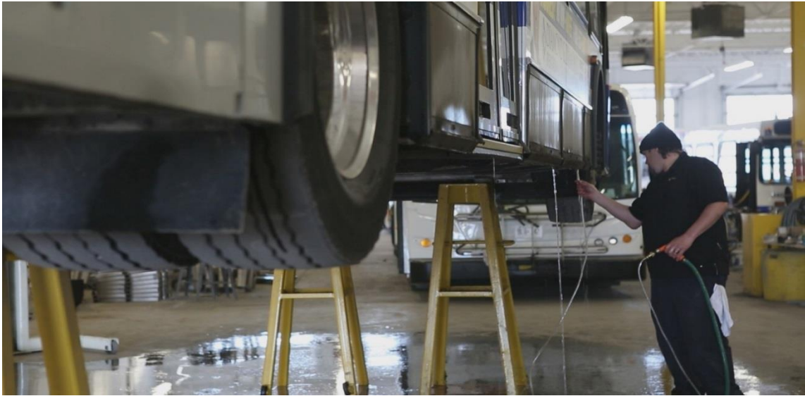
FIGURE 13: WHEN WATER COMES OUT CLEAR, THIS IS A GOOD INDICATION THAT DEBRIS AND CALCIUM HAS BEEN REMOVED FROM THE INSIDE OF THE TUBES.
