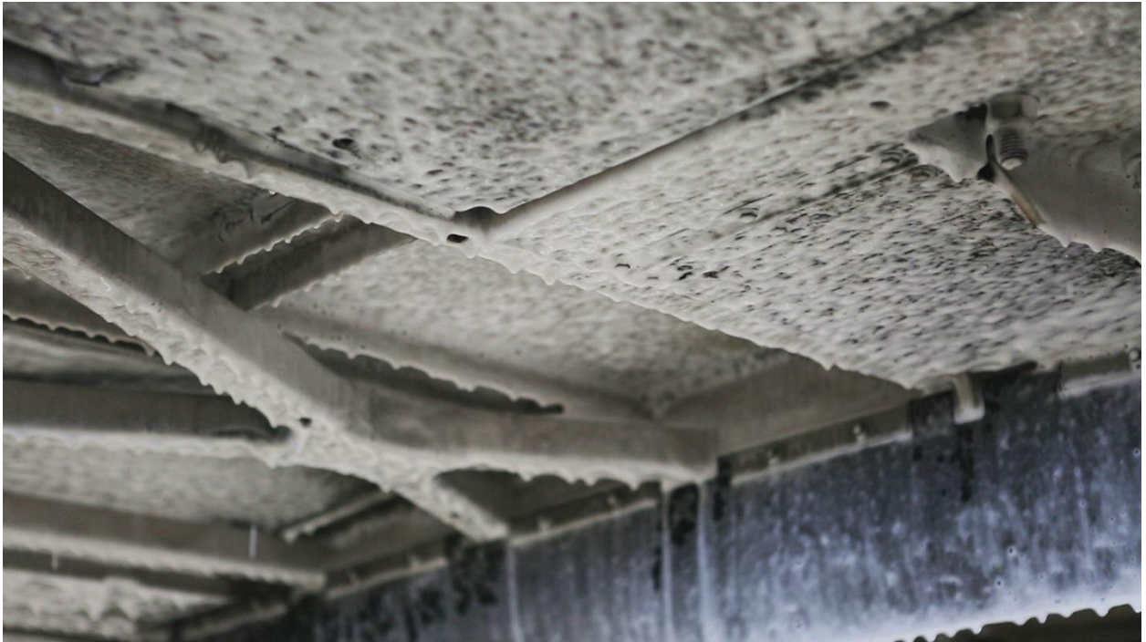
FIGURE 6: SALT ELIMINATOR APPLIED TO THE UNDERSIDE OF THE BUS.
