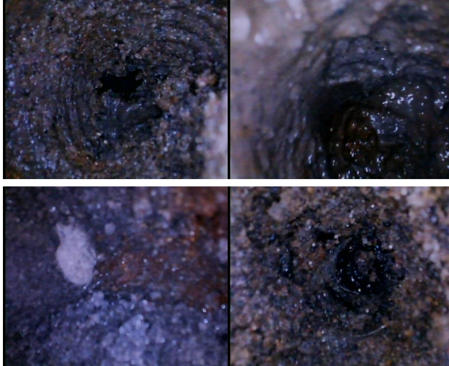
FIGURE 9: SHOWN THE DEBRIS/CORROSION INSIDE THE TUBES BEFORE TUBES ARE CLEANED AND FLUSHED OUT.
