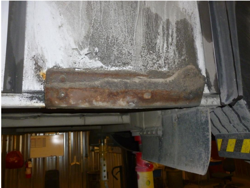
FIGURE 2A: DEBRIS BUILDUP ON LOWER IMPACT PANEL BRACKET.
