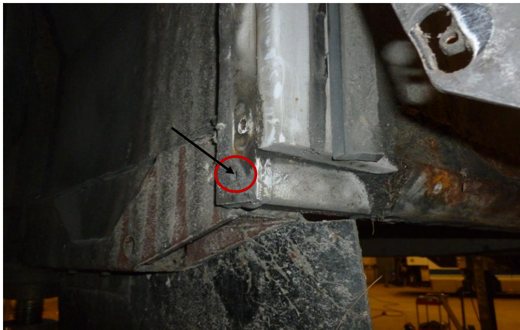
FIGURE 4B: SHOWN THE PRE-DRILLED HOLE ON THE FACE OF THE TUBE THAT WILL BE DRILLED.
