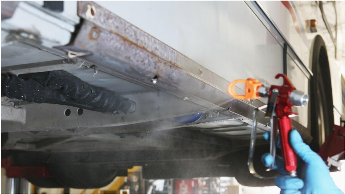
FIGURE 21: SHOWN T-40 SPRAYED AT THE LOWER IMPACT PANEL RAILS/BRACKETS
