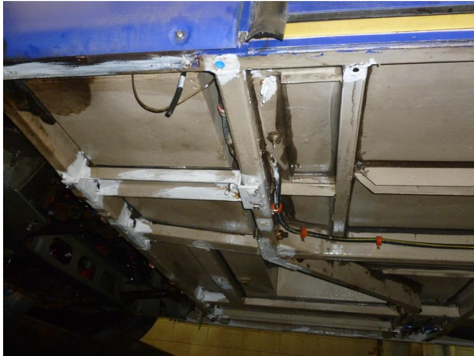
FIGURE 17: SHOWING PPG ZINC PRIMER APPLIED
