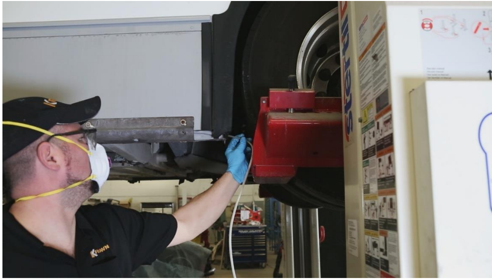
FIGURE 18: SHOWN APPLICATION OF THE T-40 INTO THE TUBES
