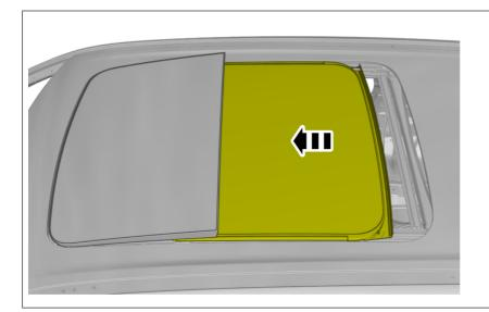
Lift the marked component forward.
