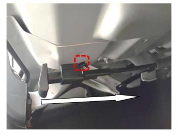
5. Using a 10mm socket, remove the 4 bolts for the right latch.
