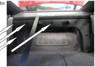
6. Using a 10mm socket, remove the 4 bolts for the left latch.
