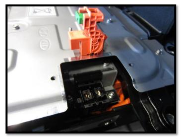
6. Remove high voltage battery cover bolts (10) using a 10mm wrench and discard the cover.
