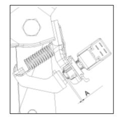
8. After replacing the stopper, check for proper function of the brake lamps. When applying the brake pedal, the brake lamps should illuminate. After releasing the pedal, the brake lamps should extinguish.
