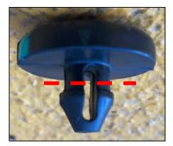
6. Install a new stopper by pressing it into place.
