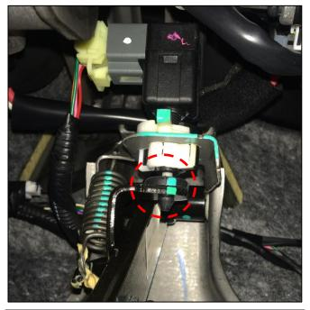
4. Remove the stopper by squeezing the engagement nub by hand, or by using pliers, and pressing the stopper out towards the stop lamp switch plunger.
