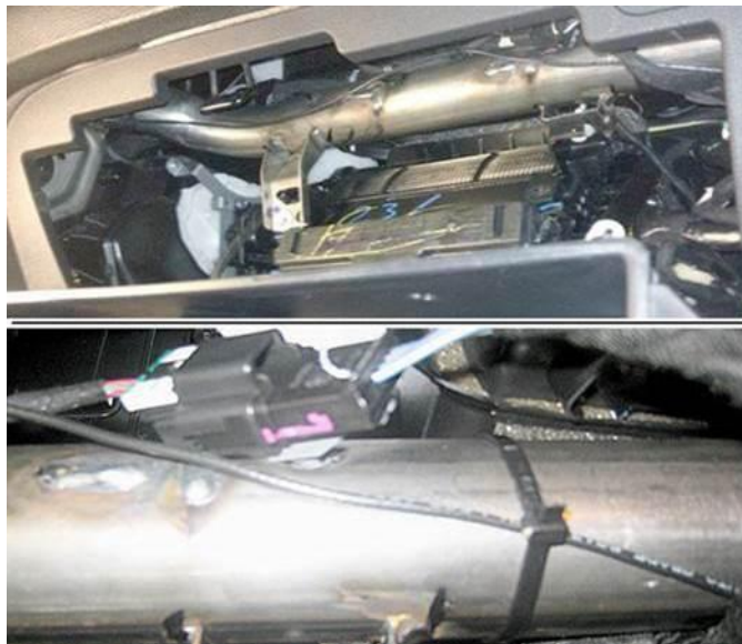
Fig. 16 IP Wiring Overlay Routing
