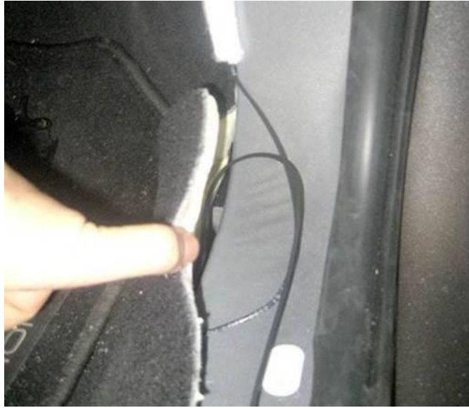
Fig. 19 IP Wiring Routing Carpet
