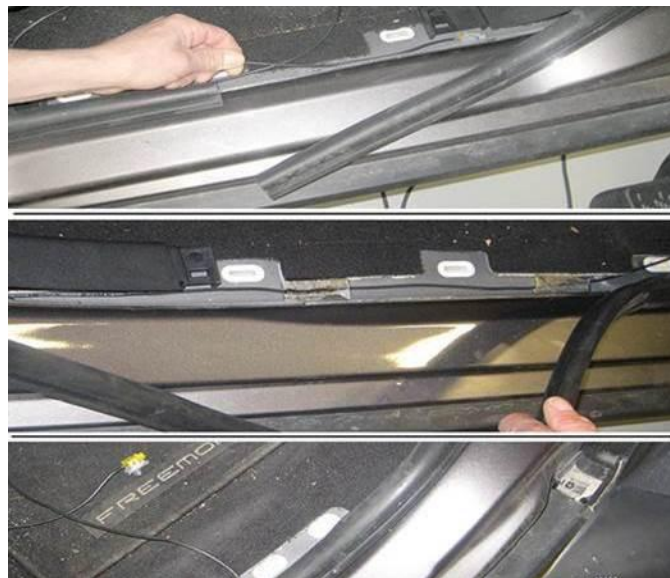
Fig. 12 Body Wiring Routing Kickplate
