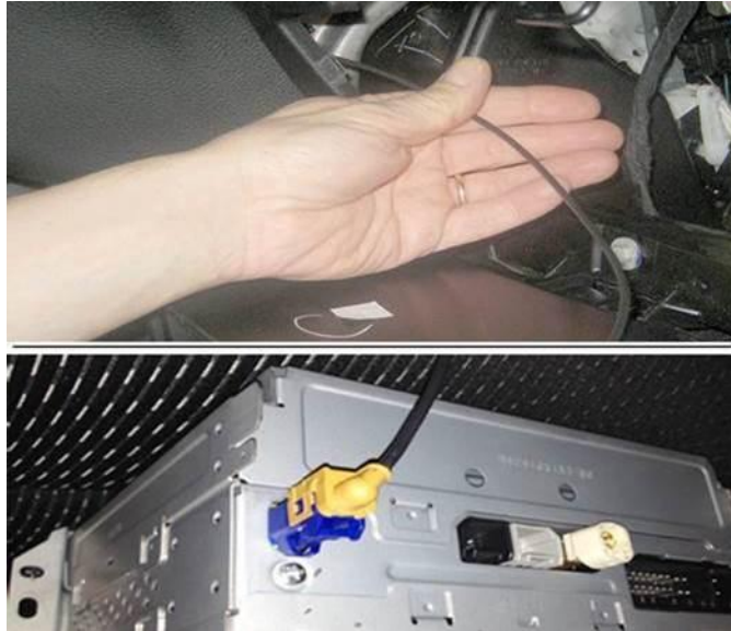
Fig. 15 GPS Connector Connection With New IP Wiring
