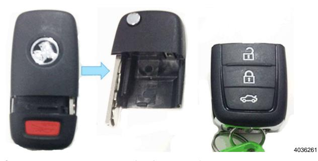
2. Separate the Remote Keyless Entry (RKE) transmitter from the key blade housing using a screw driver in the position shown.
