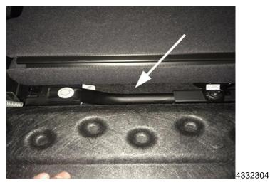
4. Identify the outboard rear cross tube of the seat assembly.
