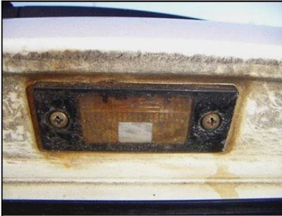
Figure 1: Corrosion on and around the license plate light
