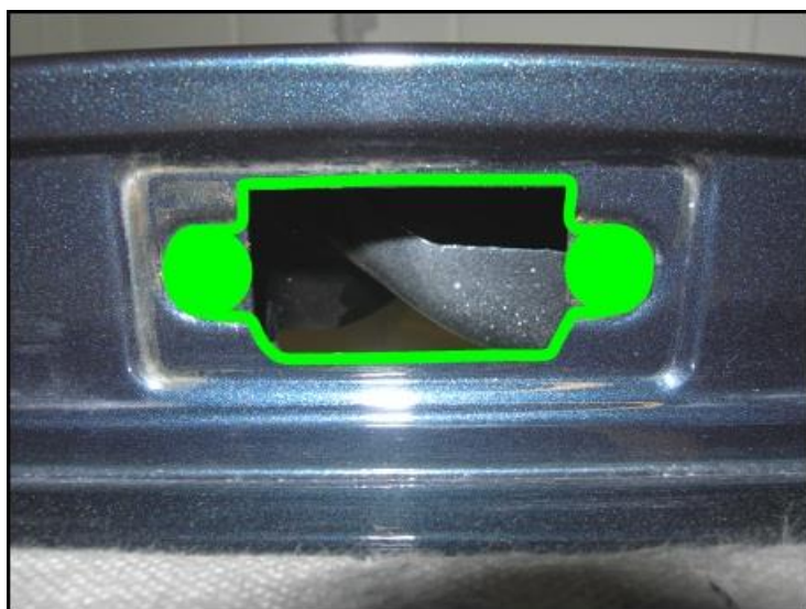
Figure 2) License plate light, butyl sealing cord areas
