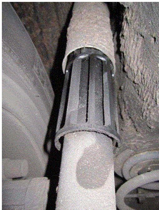
Figure 4) Not a leaking shock/strut
