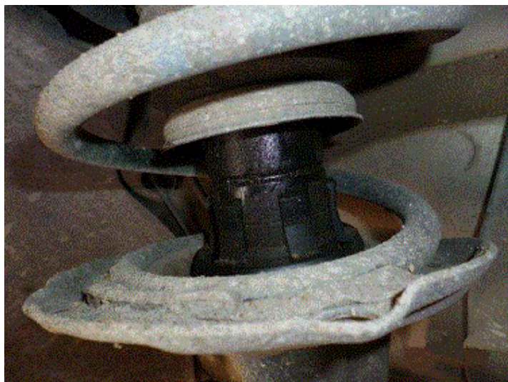
Figure 3) Not a leaking shock/strut
