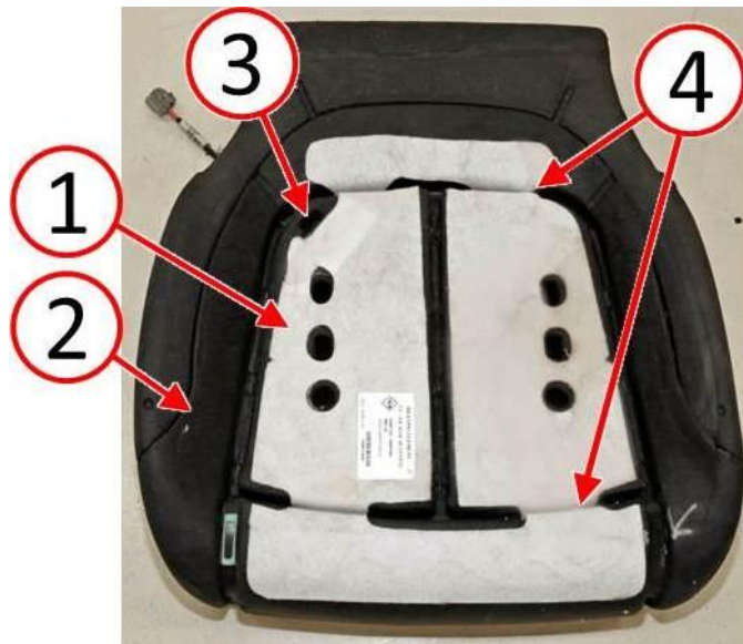
Fig. 2 Install New Heater Pad To Foam Cushion
