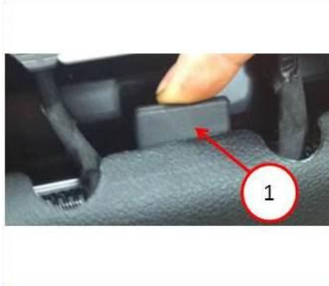
Fig. 7 Bumper Being Installed
