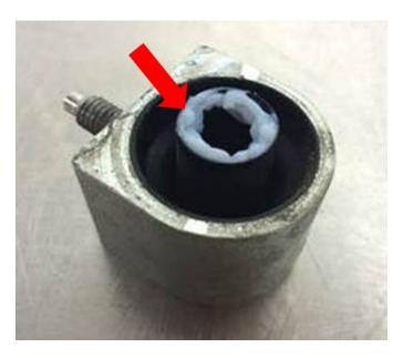
Fig. 6 Bushing Greased
