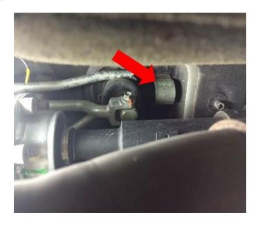
Fig. 4 Bushing On Shifter Rod
