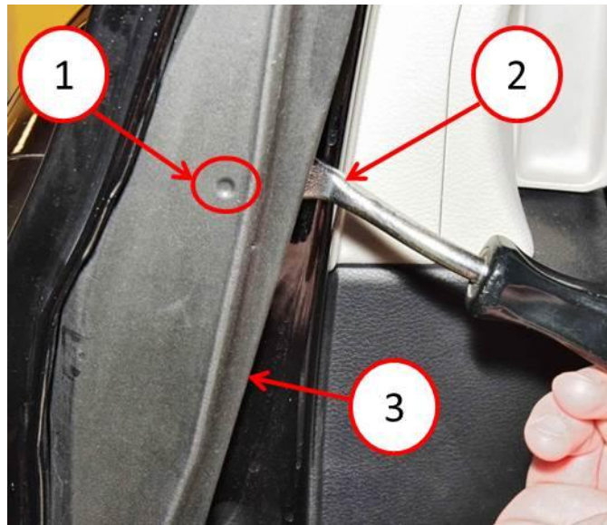
Fig. 3 Door Seal With Fasteners
