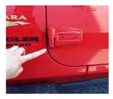
Fig. 2 Door Hinge Nut Location
