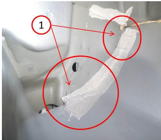
Fig. 9 Seam Not Sealed Correctly
