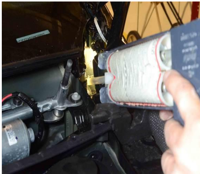
Fig. 4 Structural Adhesive At Weld Location
