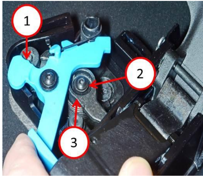
Fig. 10 Lever Opened Exposing Torx Screw
