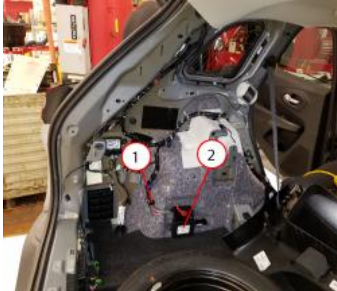
Fig. 4 Interior Trim Panels Removed For Access
