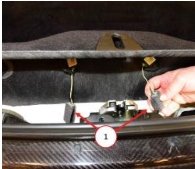
Fig. 4 Foam Tape On Electrical Connector
