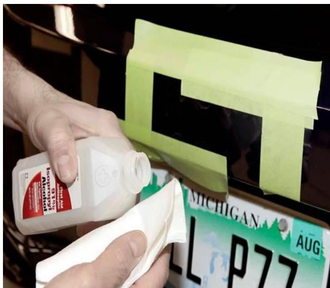
Fig. 5 Cleaning The Area
