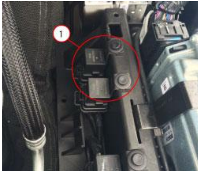
Fig. 3 Fasten Relays to Component Tray
