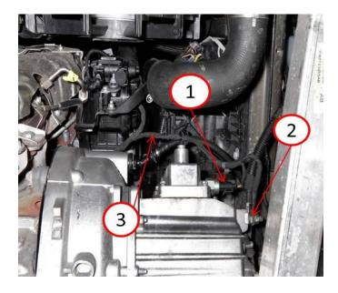
Fig. 9 Ground At Transmission
