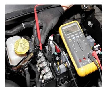
Fig. 13 Ohm Testing Fuses
