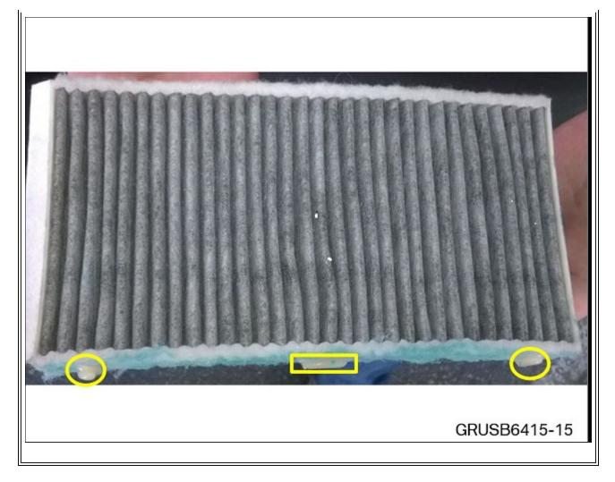
5. Allow the applied glue time to dry then then install the upper and lower micro-filters in the housing (REP 64 31 010).
