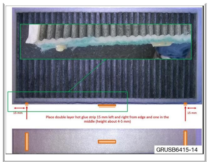
All 3 hot glue applications must be double layered, be 15 mm long and have a total height of 4-5 mm. Placement of the hot glue must in the exact locations shown to prevent complications with the condensate water flow.
