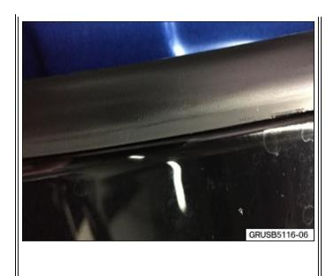
6. Use the lubricant specified below and cover the entire cover strip to prevent the door frame from sticking to the cover strip. When work is completeted, wipe off the excessive lubricant.
