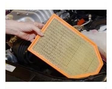
Fig. 3 Removing Air Filter
