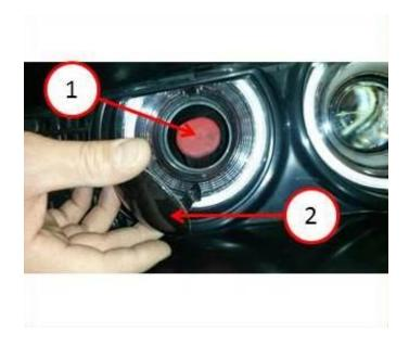
Fig. 5 Removing Air Intake Cover
