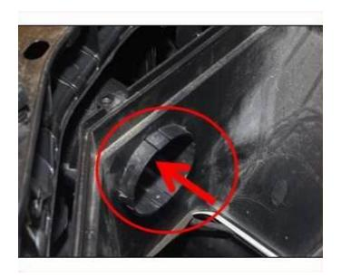
Fig. 4 Insertion Point Of Handle
