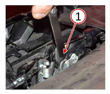
Fig. 4 Measure Hood Latch Ratchet to Latch Cover Plate Clearance
