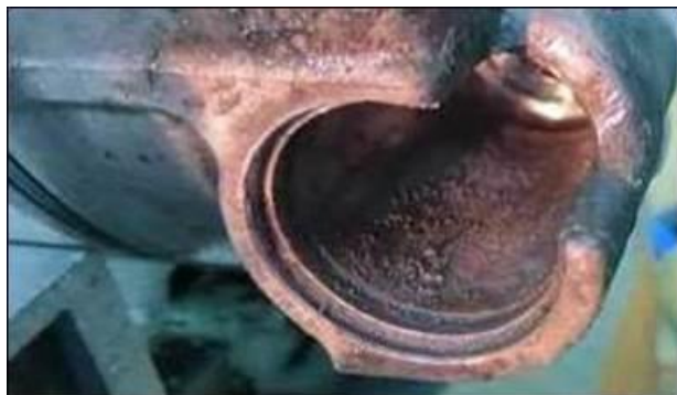
Figure 13. Corrosion in the N280 valve bore.
