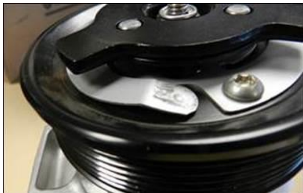
Figure 7a. Example of torque limiter over load protection activated.
