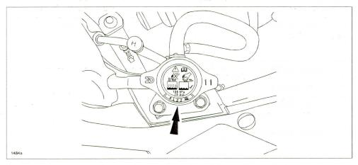
CAUTION: FL22 coolant is "pre-mixed" and must be added to the cooling system as is. **DO NOT ADD**WATER TO FL22 COOLANT. Adding water will dilute the solution and lessen the effectiveness of the coolant.
