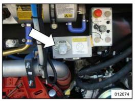
Figure 10: ELC connecting socket in engine compartment of TD925/TDX25US
